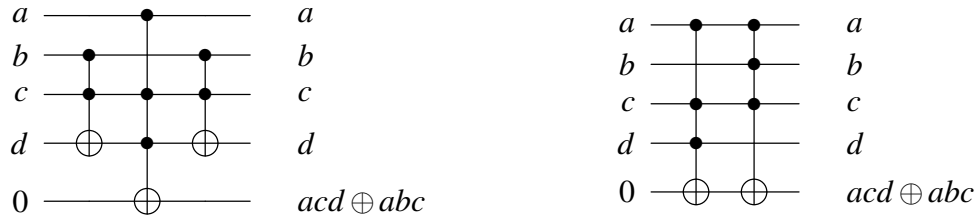
Figure 2.11: Toffoli gates for the Boolean function ( acd \oplus abc )
