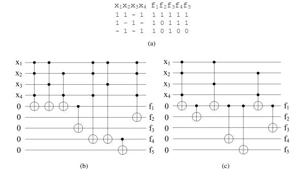
Figure 4.2: (a) An initial cube-list, (b) a Toffoli cascade generated by the approach in [46, 47], and (c) an improved Toffoli cascade.
