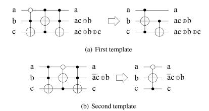
Figure 7.2: Two templates for Toffoli gates with positive and negative controls.
