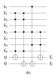
Figure 3.2: (a) An ESOP cube-list and (b) a circuit generated by basic approach.
