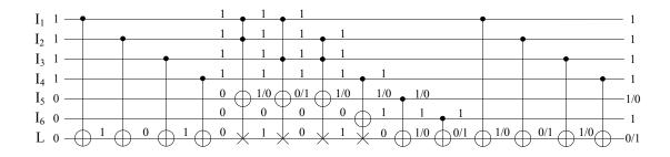
Figure 6.4: A single fault on output line  $I_5$ .
