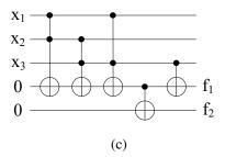
Figure 3.7: (a) An ESOP cube-list, and circuits generated (b) by basic approach with line optimization and (c) by shared cube synthesis.
