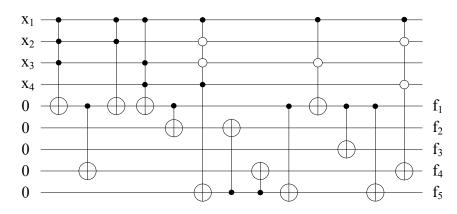
(d) A circuit equivalent to the cube-list in Figure 4.3(a).
