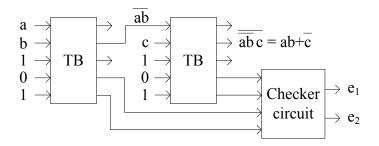
Figure 5.4: Online testable circuit for  $f = ab + \overline{c}$ , according to the design in [54, 53].
