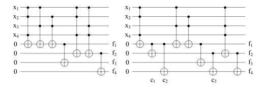
Figure 4.5: (a) An example cube-list, (b) a Toffoli cascade generated by the approach in [46, 47], and (c) a Toffoli cascade generated by our proposed approach.
