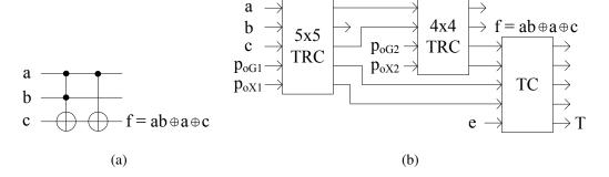
Figure 5.8: (a) A Toffoli circuit for  $f = ab \oplus a \oplus c$ , and (b) the corresponding testable circuit according to the design in [21, 22].
