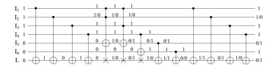
Figure 6.3: A single fault on input line  $I_2$ .
