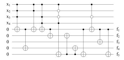
(c) Appending the circuit for sub-list<sub>3</sub> to the circuit of Figure 4.4(b).
