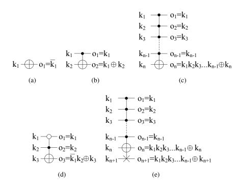
Figure 2.1: (a) A NOT gate, (b) A CNOT gate, (c) an n-bit Toffoli gate, (d) a 3-bit negative-control Toffoli gate, and (e) an (n+1)-bit ETG.
