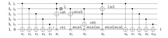
Figure 6.6: Fault detection in testable circuit.
