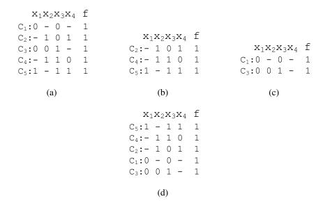
Figure 3.5: (a) Initial ESOP cube-list, (b) list 1 containing positive polarity and don't care value of  $x_1$ , (c) list 2 containing negative polarity of  $x_1$ , and (d) final reordered cube-list.
