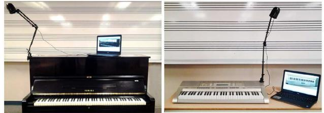
Fig. 1. Ideal location (30–45 degrees from vertical) of the camera over the piano and electronic keyboards.
