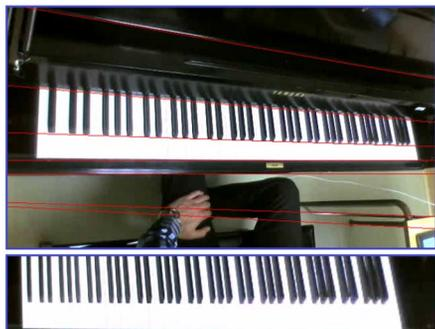
Fig. 3. Sample input image with the lines detected using Hough line transform (top) and the transformed rectangle corresponding to the keyboard in the image (bottom).
