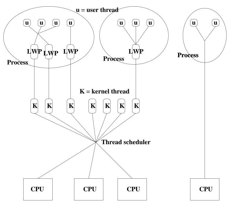
Multiple CPU system with thread scheduler, kernel threads, LWPs, and multiplexed user threads.
