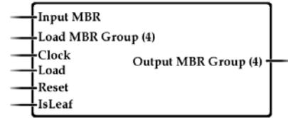
Figure 2. The input/output design for a 2\*2 node.
