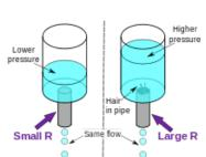
The hydraulic analogy compares electric current flowing through circuits to water flowing through pipes. When a pipe (left) is filled with hair (right), it takes a larger pressure to achieve the same flow of water. Pushing electric current through a large resistance is like pushing water through a pipe clogged with hair: It requires a larger push (voltage drop) to drive the same flow (electric current) (courtesy of wikipedia).
