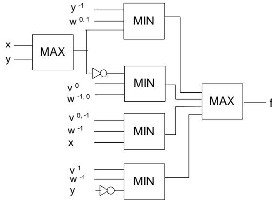
**Figure 3. A possible realization using partial (anti)symmetries for the  $n = 4$   $p = 3$  function specified in Table 2.**
